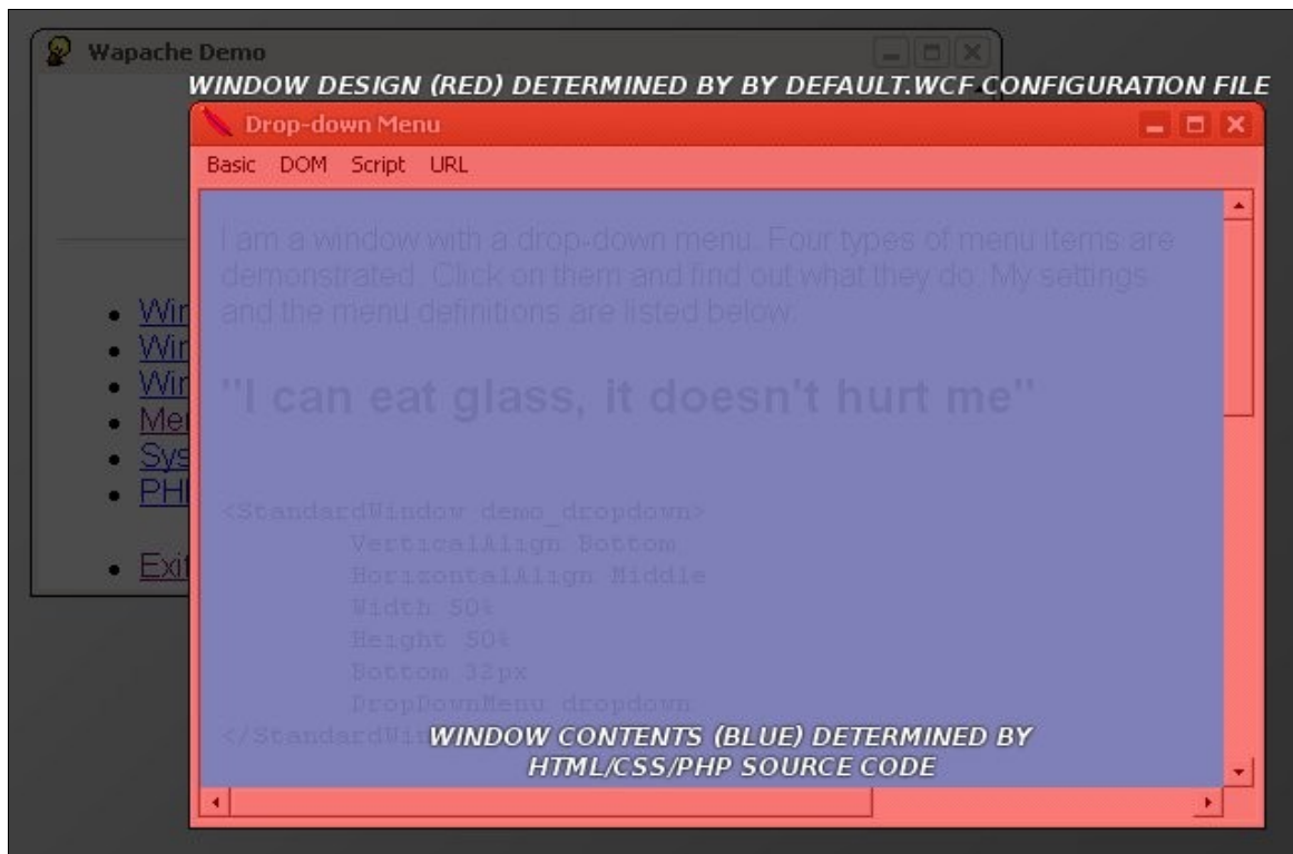
Illustration 15: A typical Wapache window. The code that determines the appearance of the application are stored in different locations. The code for the general design of the window is held in the default.wcf file, while the contents are held in the root source code folder.
